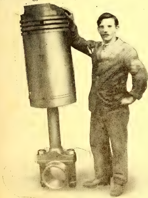
The Piston and Connecting-rod and Big-end of a Petter Two-Stroke Oil Engine.
